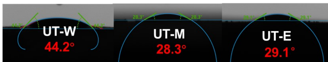
Figure S15 The water contact angle results of UT-W, UT-M, and UT-E.
