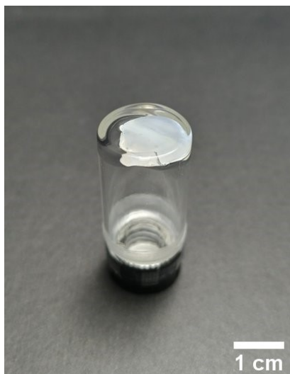
Fig. S6. Optical photograph of a pale white quasi-solid state by liquid electrolyte (1.0 M LiTFSI-DOL/DME) soaked with PSE11 over 36 hours.
