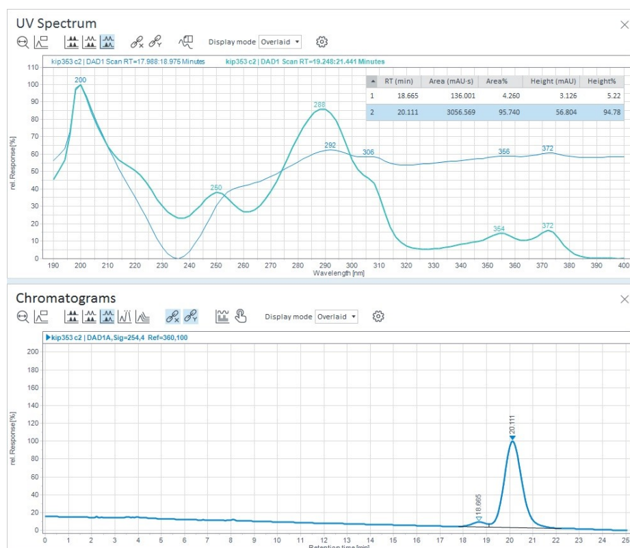
Figure S134. HPLC chromatogram of compound 5cb/diastereomer 2 (91% ee, Chiralpak IC, hexane/ i -PrOH = 90:10, 1.5 mL/min, 254 nm, t_R (major) = 20.11 min, t_R (minor)= 18.67 min).
