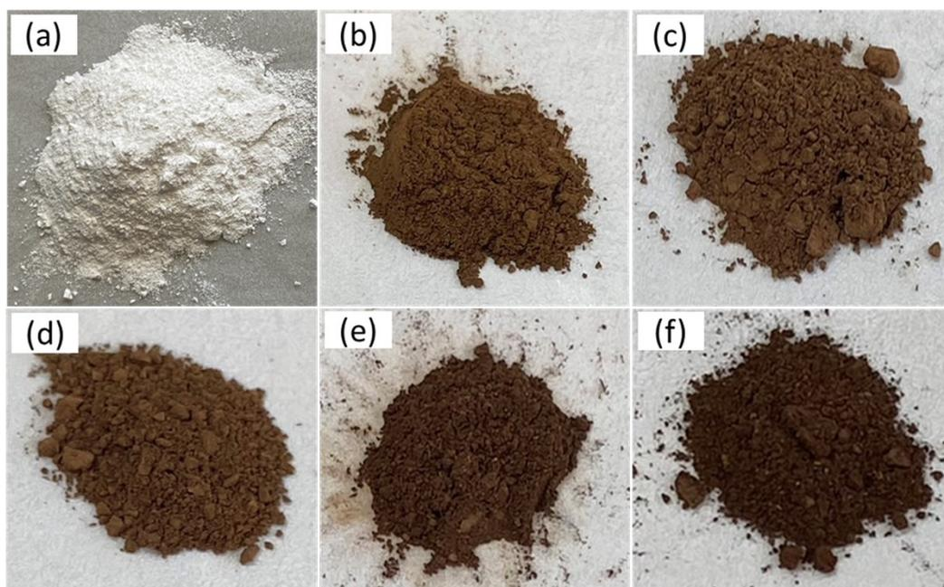
**Figure S9.** Photographs of MOF-808\* catalyst powders (a) before the reaction, and after hydrothermal reactions at 190 °C for (b) 0.5 h, (c) 1 h, (d) 2 h, (e) 4 h, and (f) 6 h, respectively.
