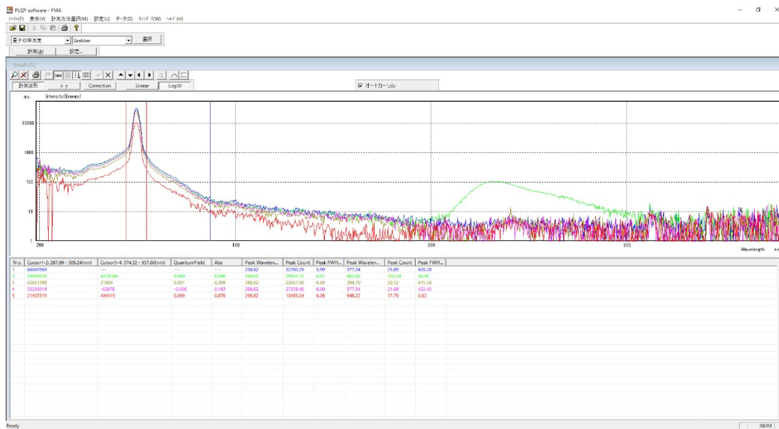
Figure S11. PL spectra of the Sb complexes and LH 3 measured by the PLQY measurement system.
