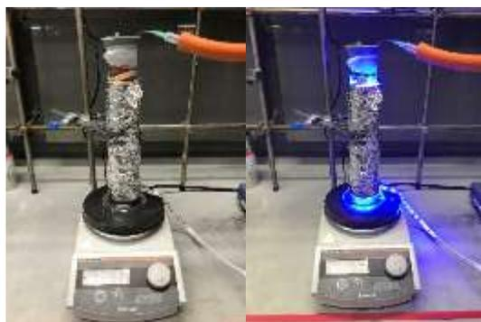
A 250 mL borosilicate glass measuring cylinder was wrapped in blue LEDs and foil, then sealed. The reactions using this set-up were conducted under a continuous flow of nitrogen.
