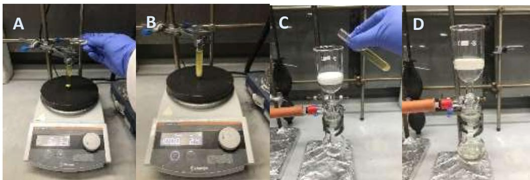
a) Addition of KF on alumina (40 wt%) to reaction mixture. b) Mixture stirred vigorously for 15 minutes. c) Mixture filtered through a short pad of silica. d) KF on alumina, excess TMS and photocatalyst do not pass into the flask below.
