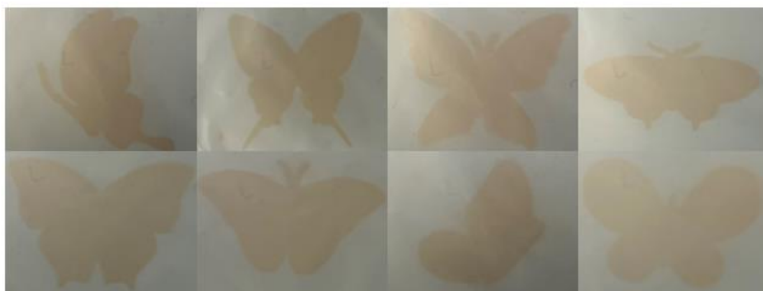
Fig. S14. Printing different patterns on 10%-iHOF-18-PVA composite membrane.
