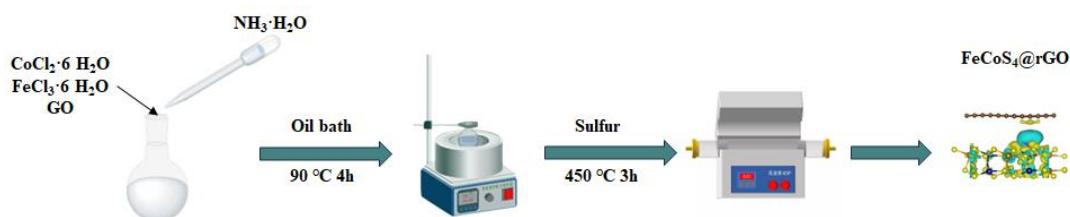
Fig. S1 Schematic illustration of the synthesis process of FeCoS 4 @rGO.
