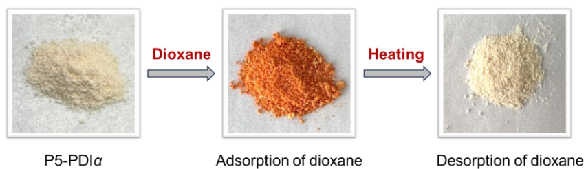
Figure S10. Color changes of P5-PDI \alpha after adsorption of dioxane and Dioxane@P5-PDI after desorption of dioxane.
