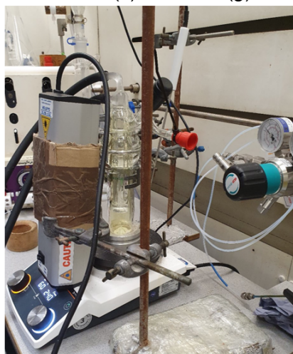
Figure S10: The apparatus with or UV photocatalysis modification to the Deville method. Note that the colour has no NO 2 character and that the N 2 O 5 condensers immediately after it has been liberated and recombined after being liberated from the silver.
