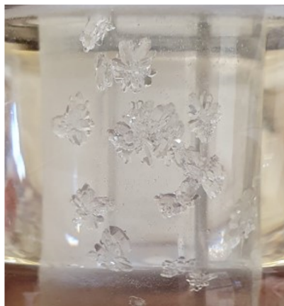
Figure S10: The apparatus with or UV photocatalysis modification to the Deville method. Note that the colour has no NO 2 character and that the N 2 O 5 condensers immediately after it has been liberated and recombined after being liberated from the silver.
