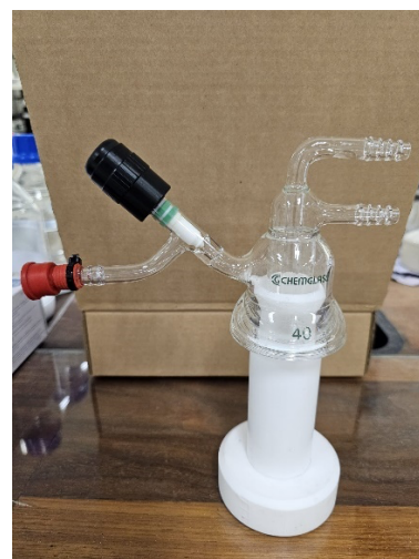
Figure S6: Assembled PTFE recovery cylinder and base with the CF inserted. Note the attached septum used for evacuating the system before priming with chlorine.
