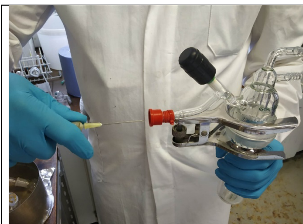
Figure S8: The needle from the high vacuum line being inserted into the septum of the CS. Note the cable tie securing the septum in place which is entirely satisfactory.
