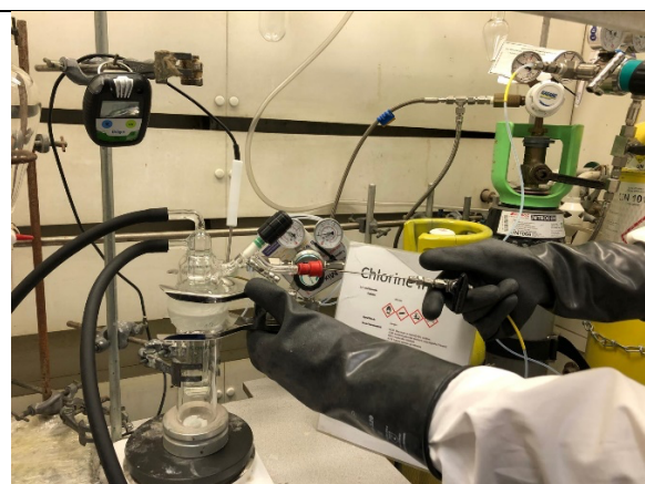
Figure S9: The evacuated CS is secured in place on the HP and the coolant lines from the chiller are attached and the chiller. The CS inlet valve is opened, then the fom the needle valve connected via PTFE tubing) is inserted into the septum. Then the valve at the needle (just below the thumb of the right hand) is opened to fill the CS with chlorine to a pressure of 0.8 bar (pressure set at the regulator). Both the valve on the needle and CS are closed and the needle withdrawn. The CS is than completely isolated from the chlorine gas supply and monitored with gas detection.
