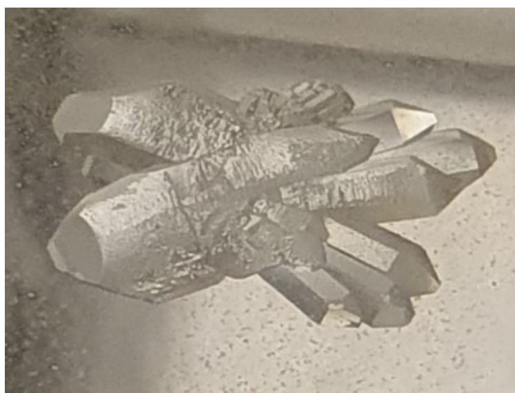
Figure S12: A close-up photograph of a dinitrogen pentoxide crystal cluster from the current work that clearly demonstrates what Deville described as “six-sided prisms which appear dependent on a right rhombus-based prism”. 1 The crystal measures approximately 1.2 cm at its longest point.
