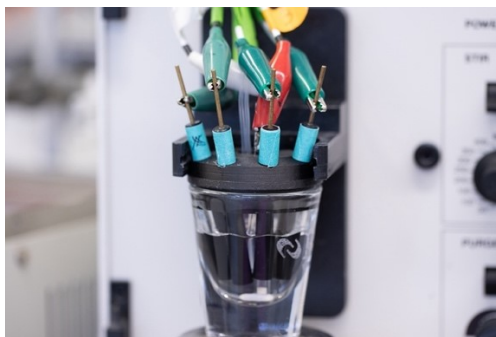
Fig S8. Photo of our electrochemical cell with 4 gold working electrodes, platinum wire and Ag|AgCl reference electrode.
