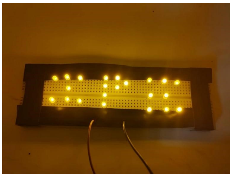
Figure S11. After MEG charges the capacitors, the series-connected LED lights forming letters can be lit directly.
