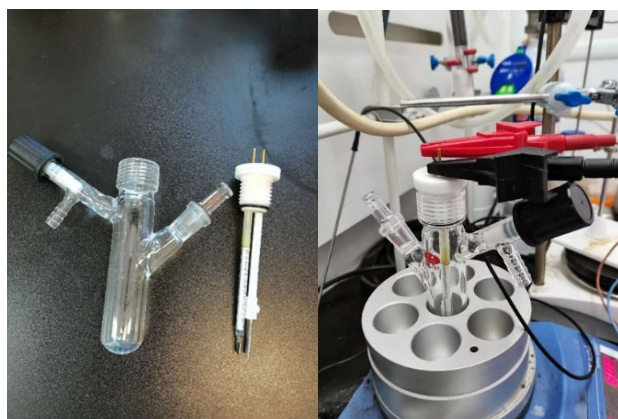
Figure S1. Photos for the electrocarboxylation. Pt (10 mm \times 10 mm \times 0.3 mm), Mg (20 mm \times 10 mm \times 0.5 mm). Electrochemical cell: 50 mL.
