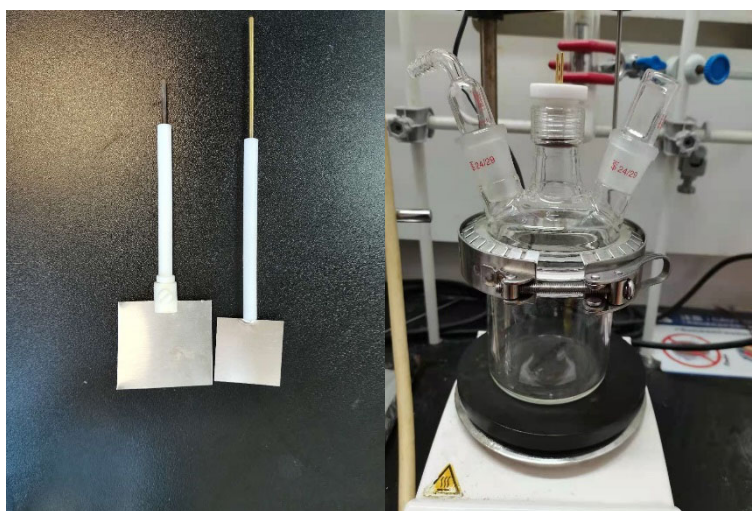
Figure S2. Photos for the gram-scale reaction. Pt 30 mm \times 30 mm \times 0.1 mm), Mg (50 mm \times 60 mm \times 0.5 mm). Electrochemical cell: 400 mL.
