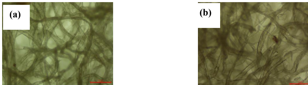
Figure S11: POM images of the (a) uncoated, (b) gel coated paper.
