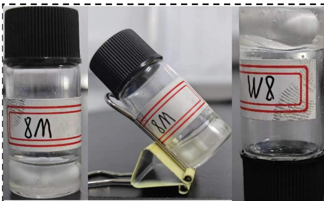
Fig. S1 Optical photos of 8 M GPE after 48 h gelation.
