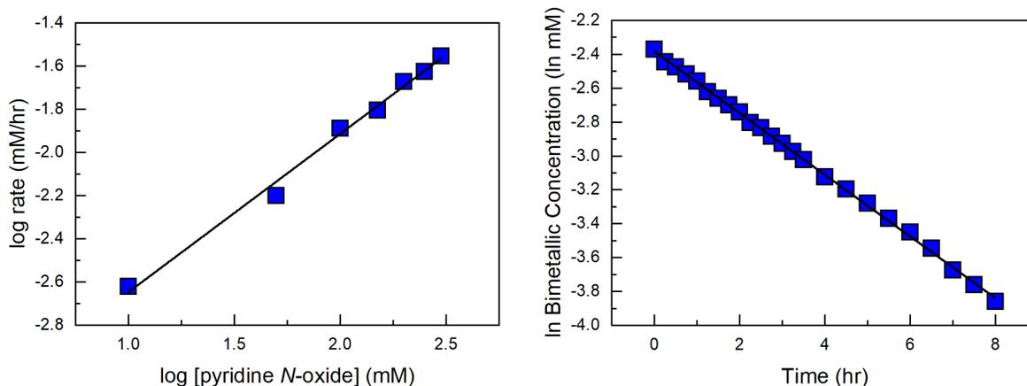
Figure S27. The log of the rate of oxidation vs the log of concentration of pyridine *N*-oxide. The linear plot shows the dependance of the reaction rate on pyridine *N*-oxide.  $y = 0.73x - 3.38$   $R^2 = 0.99$  (left) The ln of  $[\text{MoOCl}_2(\text{bpy-}^t\text{Bu})_2(\mu\text{-O})]$  concentration vs time at 100 eq of pyridine *N*-oxide. The linear plot shows the first-order dependance of the reaction rate on pyridine *N*-oxide.  $y = -0.18x - 2.38$   $R^2 = 0.99$
