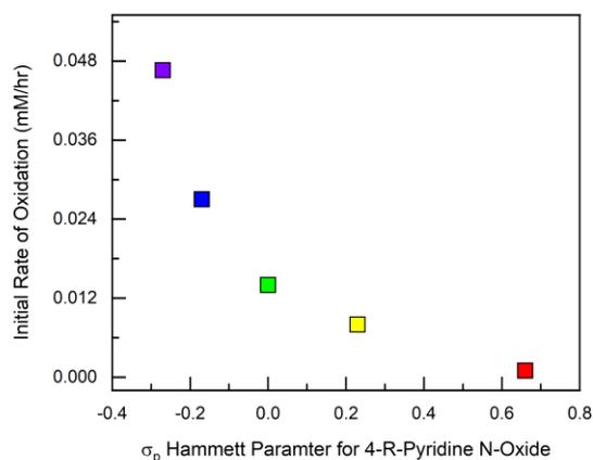
Figure S26. Hammett analysis for the initial rates of oxidation of  $[\text{MoOCl}_2(\text{bpy-}^t\text{Bu})_2(\mu\text{-O})]$  with 100 eq of a functionalized pyridine *N*-oxide. 4-*R*-Pyridine *N*-oxides used: R= OCH<sub>3</sub> (purple), CH<sub>3</sub> (blue), H (green), Cl (yellow), CN (red)
