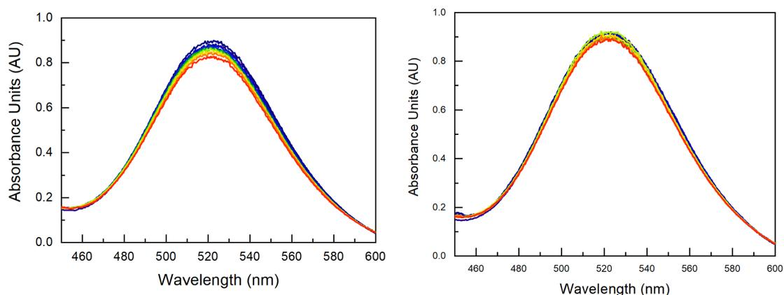
Figure S28. The UV-Vis of  $[\text{MoOCl}_2(\text{bpy-}^t\text{Bu})_2(\mu\text{-O})]$  with 10 eq of pyridine *N*-oxide and 1 eq of TPPCl (left). The UV-Vis over time of  $[\text{MoOCl}_2(\text{bpy-}^t\text{Bu})_2(\mu\text{-O})]$  with 10 eq of lutidine *N*-oxide and 1 eq of TPPCl (right). UV-Vis spectra shown in 1h increments from 0 min (purple) to 8 h (red)
