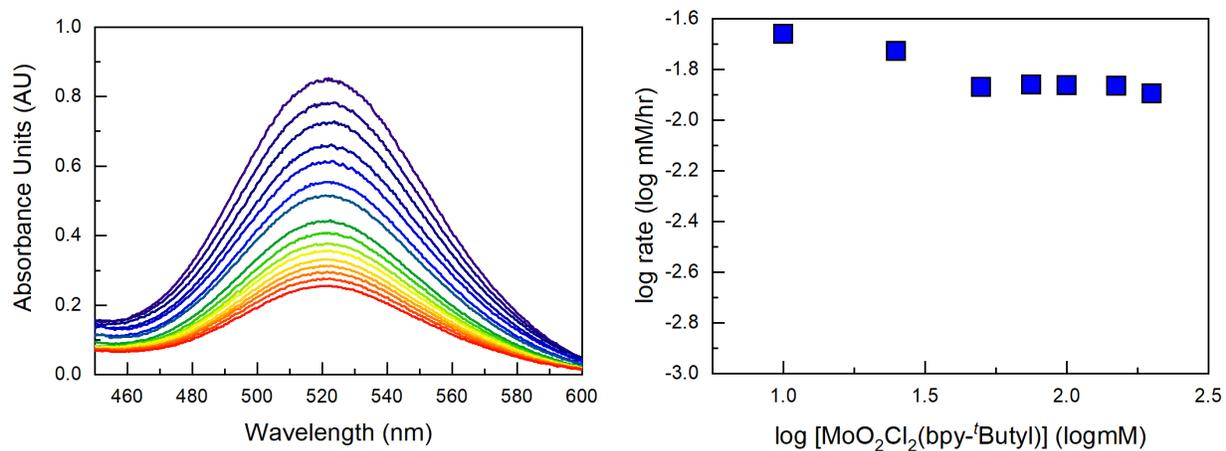
Figure S30. UV-vis over time of  $[\text{MoOCl}_2(\text{bpy-}^t\text{Bu})]_2(\mu\text{-O})$  with 100 eq of pyridine N-oxide and 100 eq of  $\text{MoO}_2\text{Cl}_2(\text{bpy-}^t\text{Bu})$ . UV-Vis spectra shown in 30 min increments from 0min (purple) to 8h (red) (left) The log plot of the oxidation rate when varying the concentration of  $\text{MoO}_2\text{Cl}_2(\text{bpy-}^t\text{Bu})$  (right).
