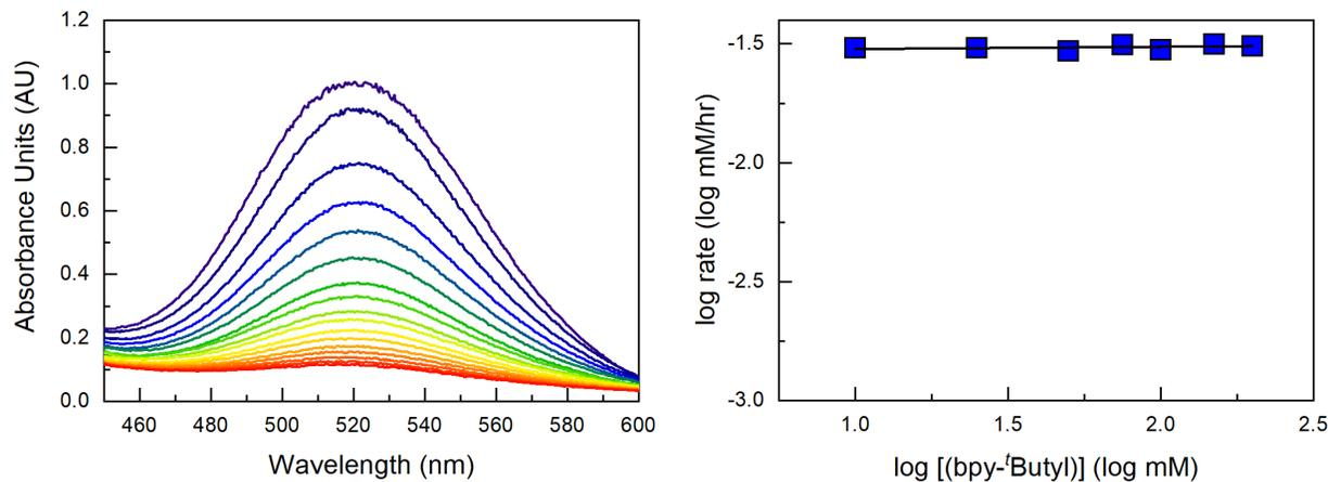
Figure S29. UV-Vis over time of a  $[\text{MoOCl}_2(\text{bpy-}^t\text{Bu})]_2(\mu\text{-O})$  solution with 100 eq of pyridine *N*-oxide and 100 eq of  $\text{bpy-}^t\text{Bu}$ . UV-Vis spectra shown in 30min increments from 0 min (purple) to 8h (red) (left) The log plot of the oxidation rate when varying the concentration of the bipyridine ligand  $y = 0.0095x - 1.53$   $R^2 = 0.16$  (right)
