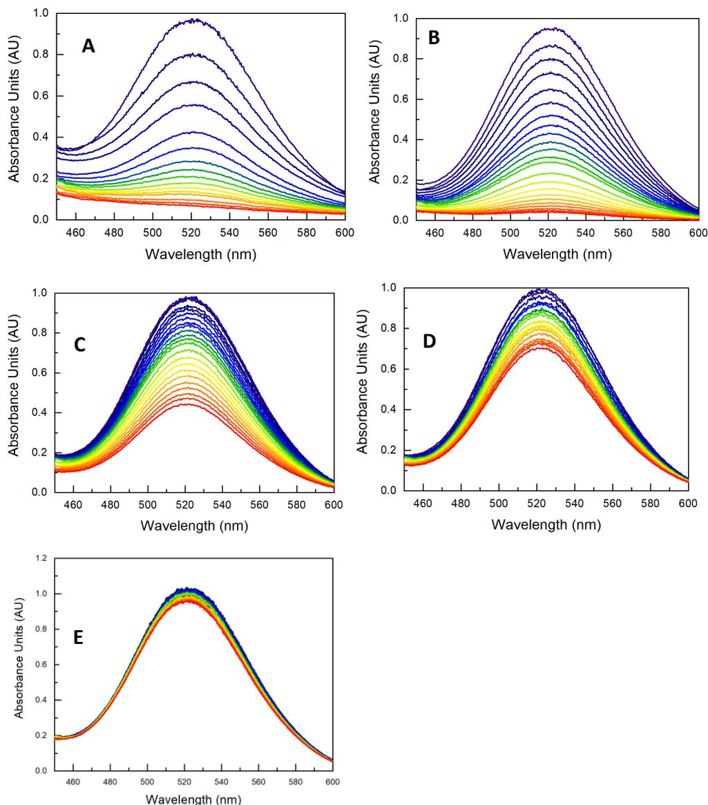
Figure S25. The UV-vis spectra of oxidation of  $[\text{MoOCl}_2(\text{bpy-}^t\text{Bu})_2(\mu\text{-O})]$  with 100 eq of a functionalized pyridine *N*-oxide. Spectra are shown in 30 min increments with 0 min in purple and 8 h in red. (A) OMe pyridine *N*-oxide (B) Me pyridine *N*-oxide (C) Cl pyridine *N*-oxide (D) lutidine *N*-oxide (E) CN pyridine *N*-oxide
