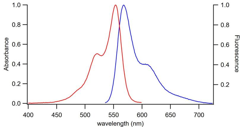
**Figure S6.** Excitation and emission spectra of AF555.
