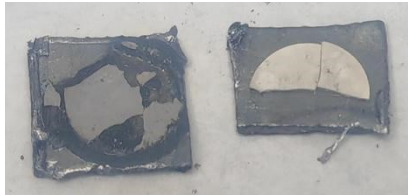
Fig. S5 optical photograph of KCl-CaH 2 mixture after heated at 600 °C (left) and 400 °C (right) for 2 h, respectively. We press the mixture into a disk under 10 MPa, and the support is graphite. The picture shows that the mixture has no signal of melting under 400 °C, while obviously melting at 600 °C.
