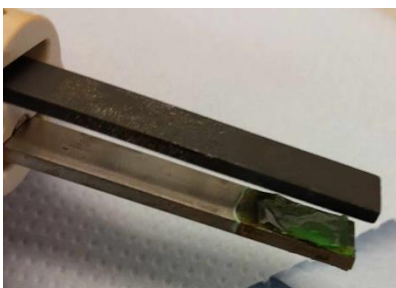
Figure S25: Black and green plated deposits on the stainless steel electrode (cathode)
