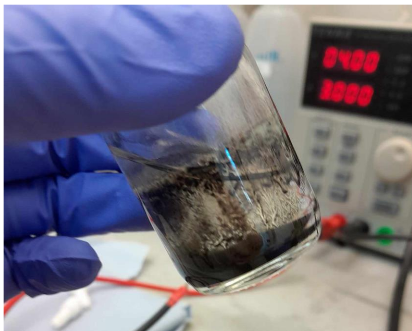
Figure S23: ElectroReact reaction mixture containing a biphasic and a large quantity of black particulate matter.
