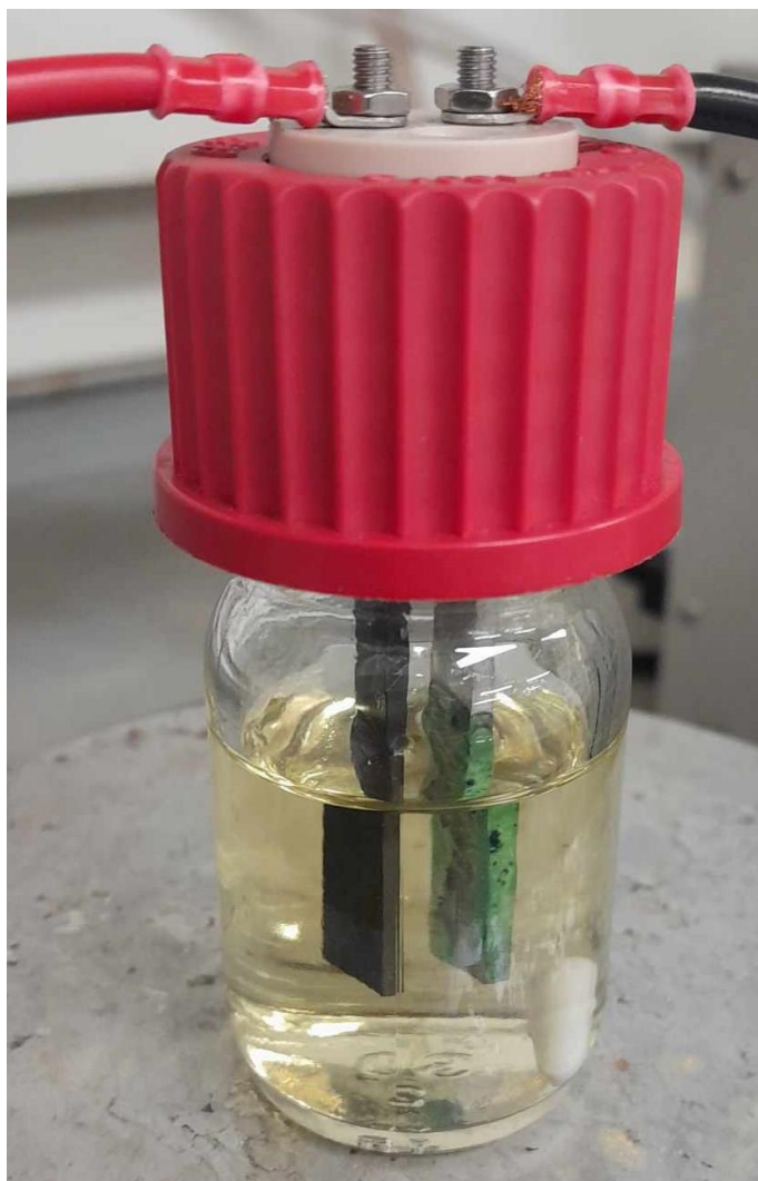
Figure 1: Reaction after electrochemical recovery (DRH-04-58-4). Note the green Ni compounds deposits alongside the black spots, possibly of Ni nanoparticles.
