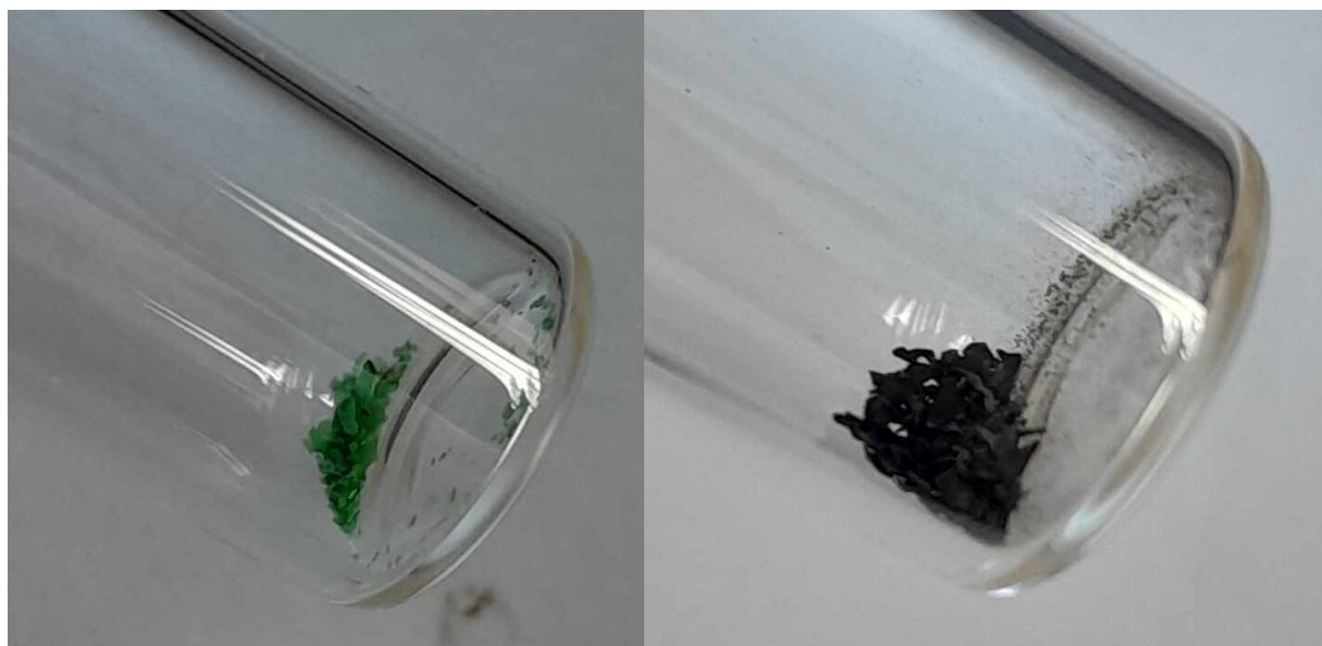
Figure S34: (left) sample of powdered Ni flakes (anaerobic) before drying, (right) sample of powdered Ni flakes (anaerobic) after drying
