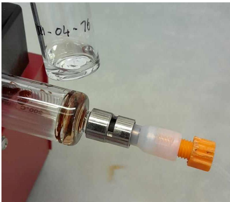
Figure S47: \text{NiCl}_2(\text{dppp}) solution in 1,4-dioxane/ \text{H}_2\text{O} before (bottom) and after (top) electrolysis.
