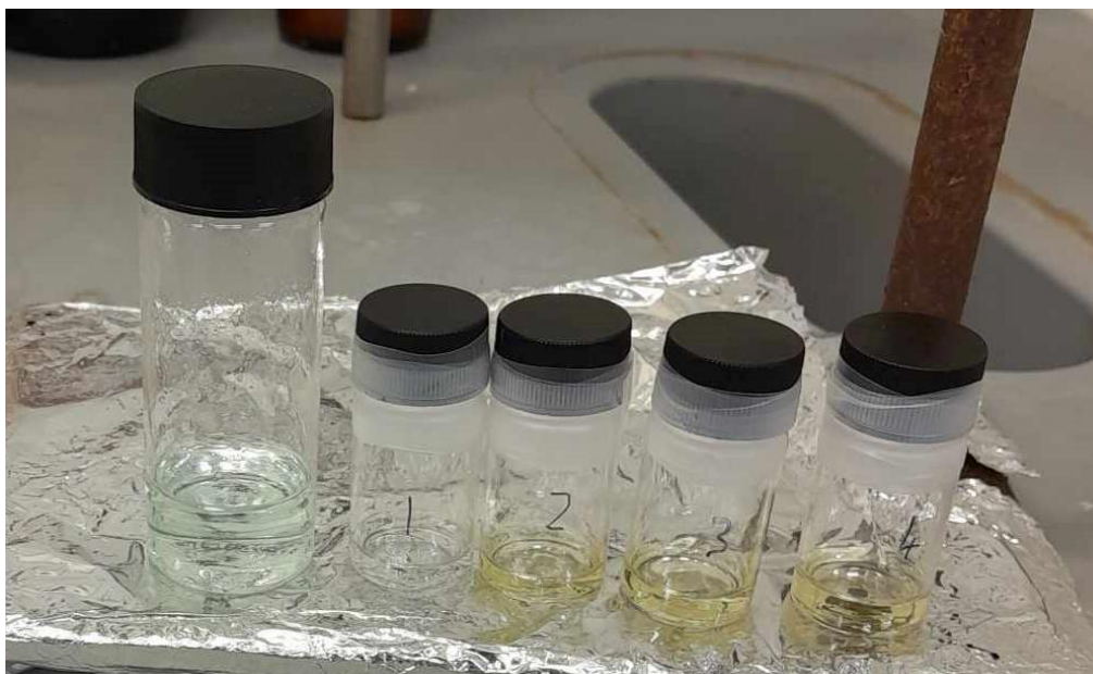
Figure S42: Solutions of \text{NiBr}_2(\text{PPh}_3)_2 in \text{MeCN}/\text{H}_2\text{O} . Stock solution before electrolysis (left), then collections throughout the reaction. Note the increasing yellow of the collected samples likely due to the generation of \text{Br}_2 in solution.
