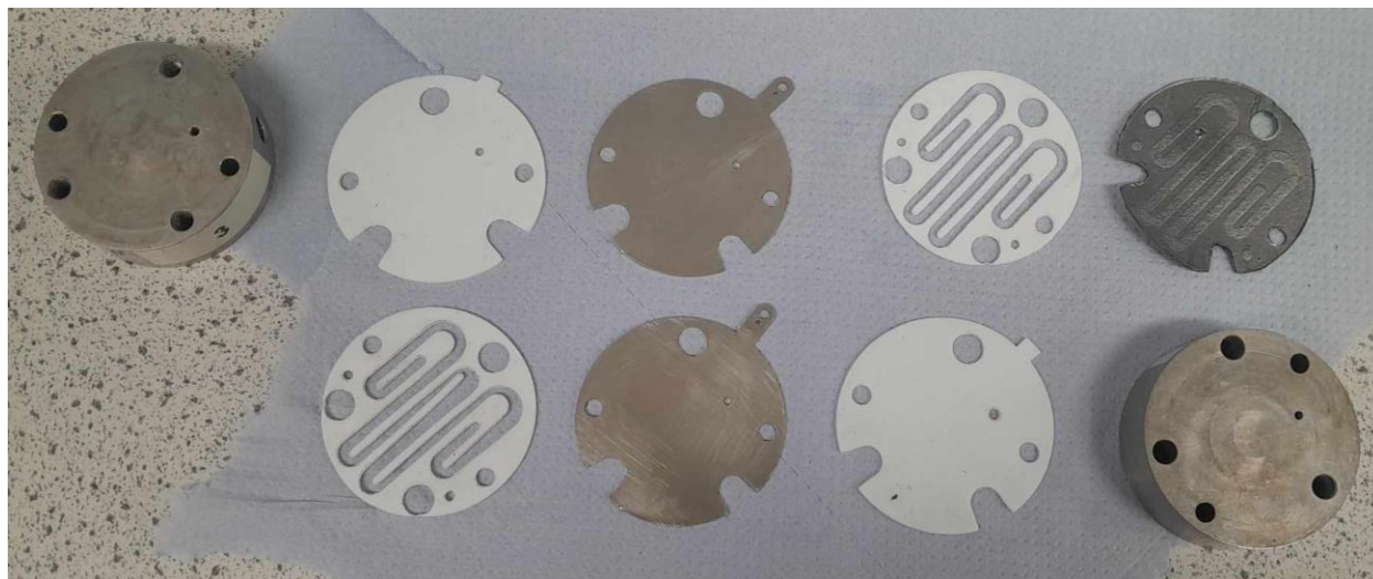
Figure S36: Reactor components. 2x stainless steel (SS) electrodes and 1x graphite electrode. 2 PTFE spacers (1 mm thickness) were used, each with a flow channel volume of 0.464 mL. This gave an overall reactor volume of 0.928 mL.
