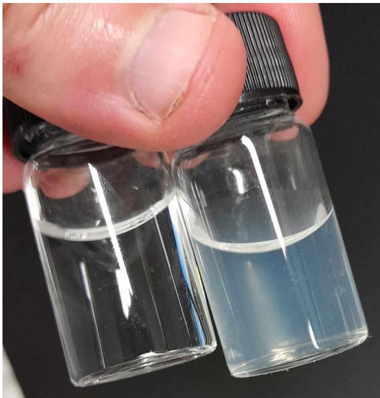
Figure S31: (left) \text{AgNO}_3 solution, (right) \text{AgNO}_3 solution after addition of supernatant from powdered Ni flakes sample. Note the light turbidity indicating the presence of bromide ions (as AgBr).
