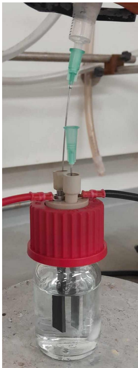
Figure S32: Electrochemical recovery setup (using quantities from Section 8.3) under a flow of N_2
