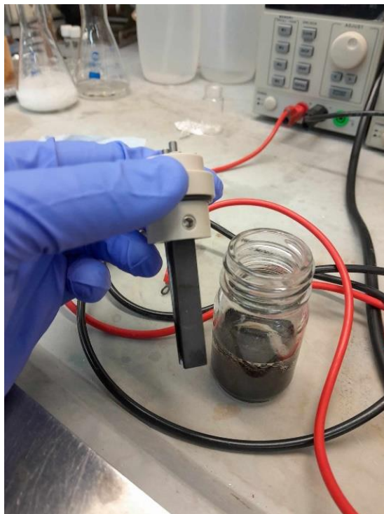
Figure S21: Graphite electrode (anode) and reaction mixture from the ElectroReact.
