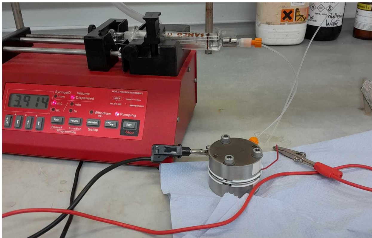
Figure S39: Syringe pump and flow reactor.
