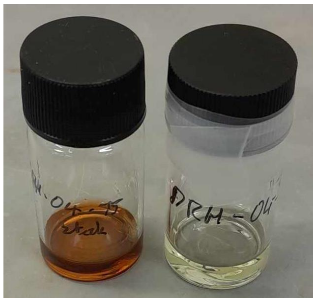
Figure S45: \text{NiCl}_2(\text{dppp}) solution before (left) and after (right) electrolysis.
