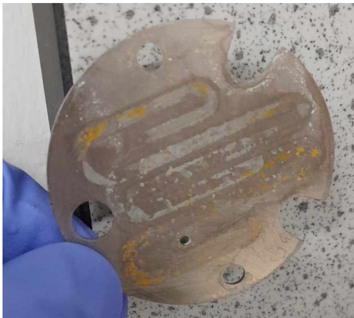
Figure S46: Stainless steel (+ve) electrode after electrolysis. Note the orange flakes of Ni compounds deposited along the flow pathway.
