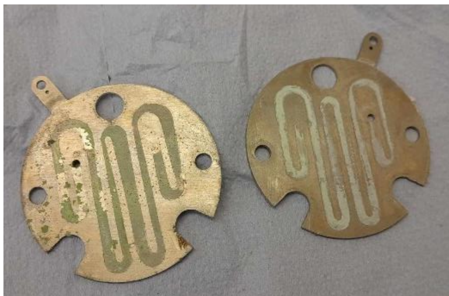
Figure S43: Stainless steel electrodes (cathode) showing green deposits of Ni metal following the reaction channel.
