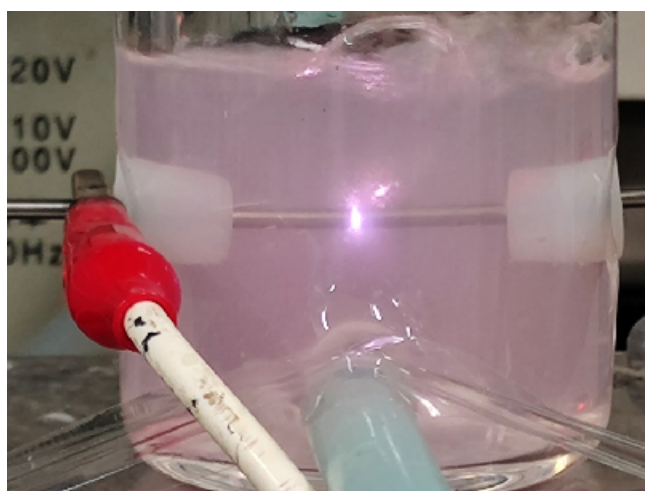
Figure S4. Pictures of the solution during discharge with the addition of 1 mmol \text{Co(OH)}_2 .
