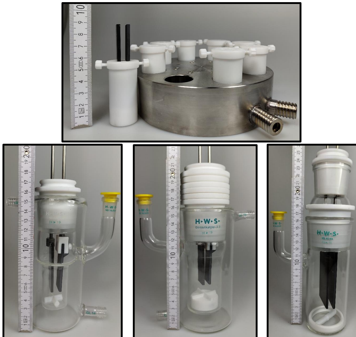
Figure S3: Different batch-type cells; size compared to a ruler: top: 5 mL undivided Teflon™ screening cells with glassy carbon and BDD electrodes and screening cell holder with integrated radiator loop; bottom left: 25 mL undivided glass cell with glassy carbon and BDD electrodes; bottom centre: 100 mL undivided glass cell with glassy carbon and BDD electrodes; bottom right: 300 mL divided glass cell with glassy carbon and BDD electrodes.
