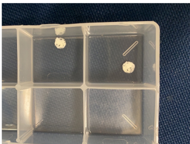
Fig S3. a) and b) Mesoporous CeO 2 samples for the USAXS/WAXS experiment. The powder is in between two transparent sapphire windows. c) Linkam 1500 thermal stage.
