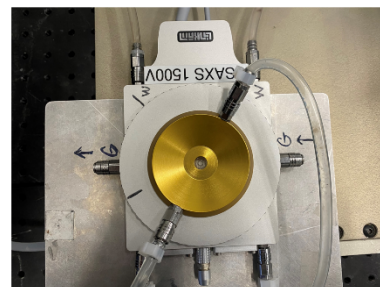
Fig S3. a) and b) Mesoporous CeO 2 samples for the USAXS/WAXS experiment. The powder is in between two transparent sapphire windows. c) Linkam 1500 thermal stage.
