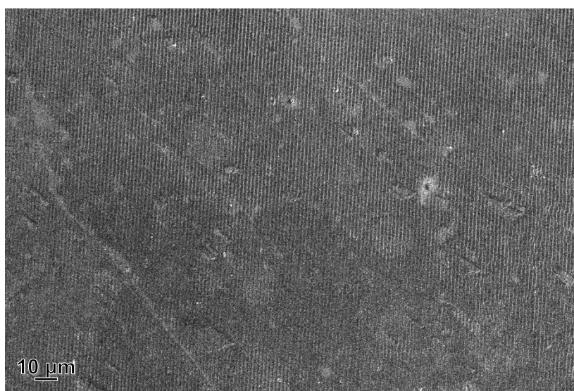
Fig. S3 A representative large-scale SEM image of TMP-grafted HOPG micropatterned by MCIL using 1.5 \mu\text{m} PDMS linear grating.
