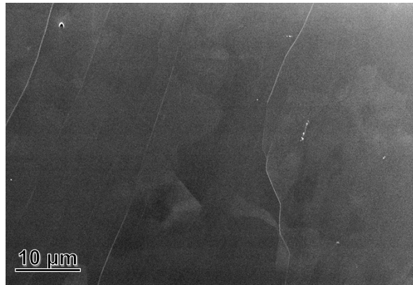
Fig. S1 A representative SEM image of TMP-grafted HOPG surface after an attempted MCIL using a hard polycarbonate grating with a pattern periodicity of 1.5 μm. This image demonstrates the absence of patterned features, underscoring the ineffectiveness of the hard stamp in achieving microscale patterning on the HOPG surface.
