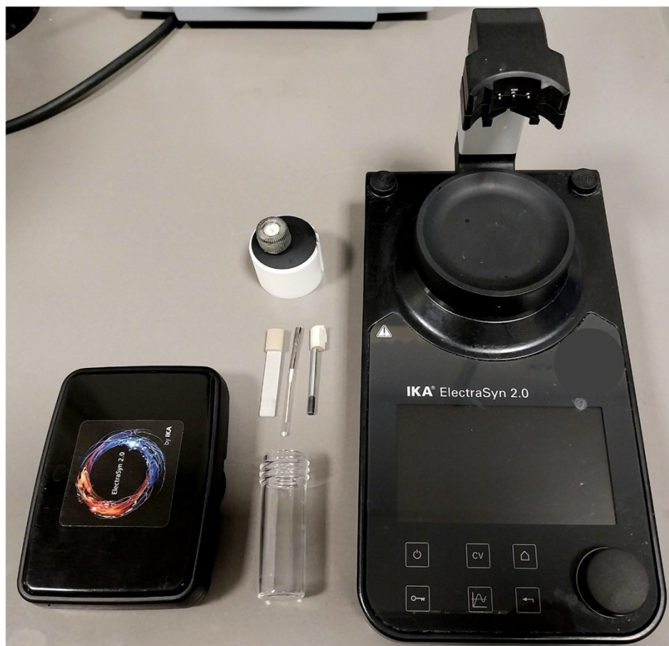
Figure S1. Electrasyn 2.0 and cyclic voltammetry set of electrodes used for collecting the voltammograms.
