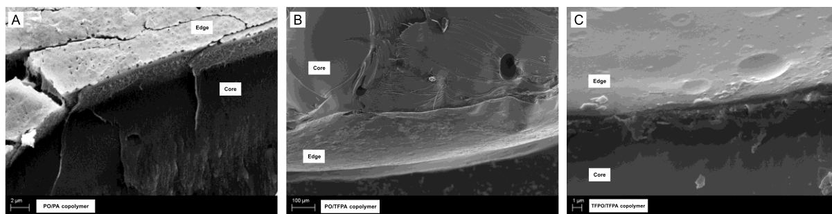
Supplementary Figure 61 - SEM images of cross-section of polymer films after degradation in 5 wt.% NaOH 6:4 EtOH:H 2 O hydrolysis solution at 40 °C.
