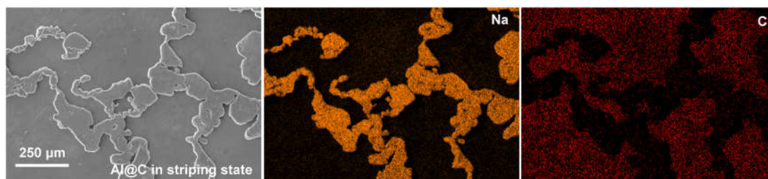
Figure S12. The anode-side SEM image and the corresponding EDS mappings of Al@C||NVP cell after 100th cycle at 100 \text{ mA g}^{-1} in a fully discharged state.
