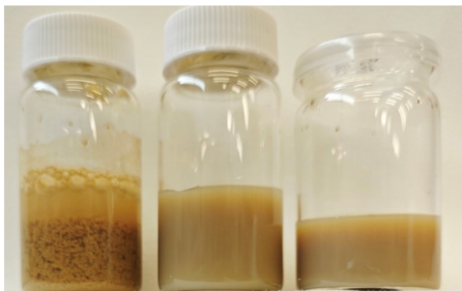
Fig. S2. 0.05 wt.% SiNWs aqueous suspensions at pH 3.6, 7.0 and 10.4 (respectively).
