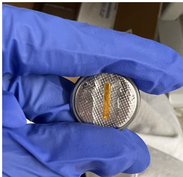
Figure S10. Photograph of the customized CR2016 cell used for the operando XRD measurement in transmission geometry. A rectangular slit ( 10\text{ mm} \times 2\text{ mm} ) was cut on both the top and bottom cases to allow for the transmission of the X-ray. The slit was sealed by a Kapton film from the inside and epoxy glue from the outside of the cell case.
