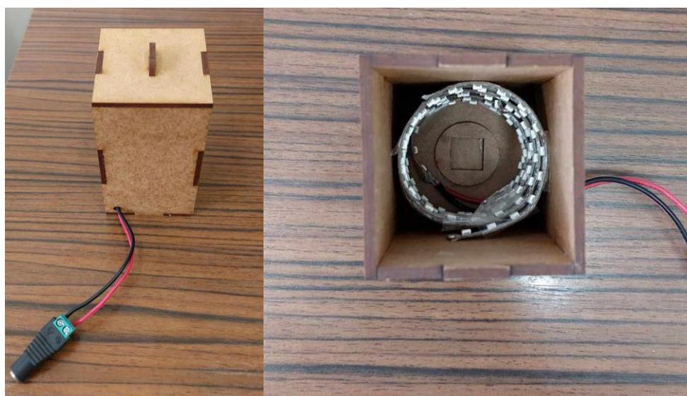
Figure S2: Irradiation box equipped with 400 nm LED strip.
