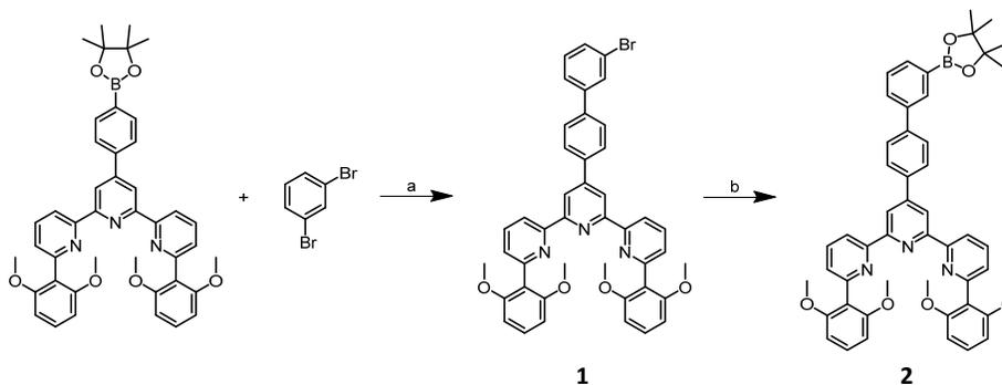
**Scheme S2.** Synthesis of **1** and **2**. *Reagents and conditions:* (a) Pd(PPh<sub>3</sub>)<sub>4</sub>, K<sub>2</sub>CO<sub>3</sub>, toluene/H<sub>2</sub>O/*t*-BuOH (3/3/1, v/v/v), reflux; (b) bis(pinacolato)diboron, Pd(dppf)Cl<sub>2</sub>, KOAc, 1,4-dioxane, 80 °C.
