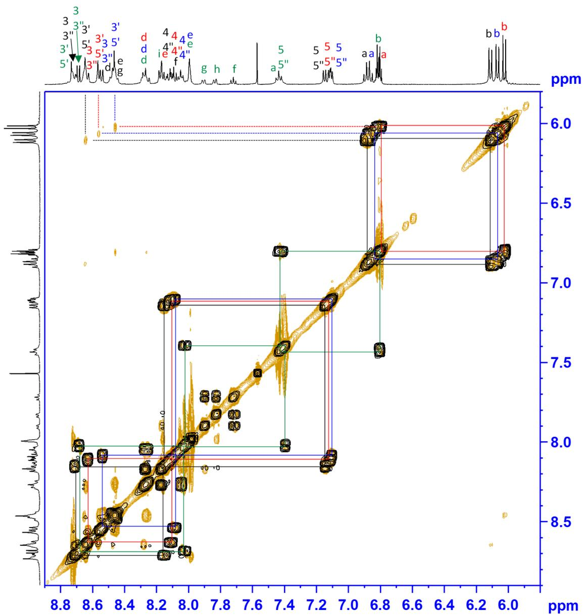
**Figure S19.** Partial ROESY NMR spectrum of  $ML^1$ . (yellow: ROESY signals, black: COSY signals).
