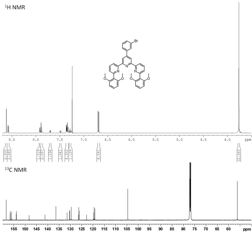
**Figure S4.**  $^1\text{H}$  and  $^{13}\text{C}$  NMR spectra of  $\text{L}^1$ .
