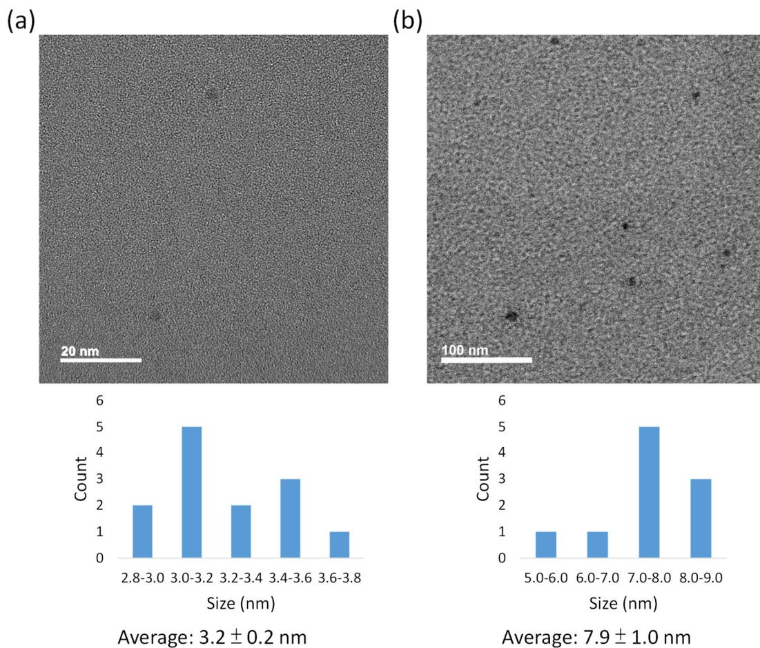
**Figure S40.** TEM images of (a)  $C^1$  and (b)  $C^2$ , and the statistical analysis for the diameters.
