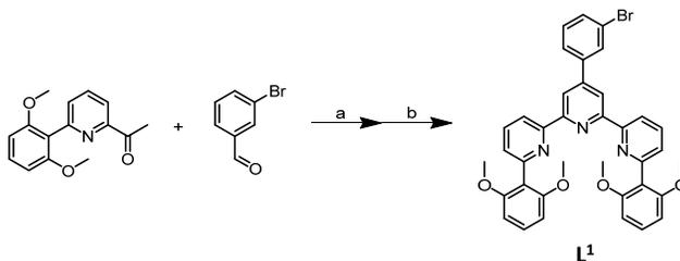
**Scheme S1.** Synthesis of L<sup>1</sup>. *Reagents and conditions:* (a) NaOH, MeOH, 25 °C; (b) NH<sub>4</sub>OH(aq), reflux.
