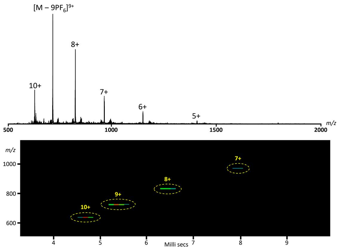
Figure S32. ESI-MS spectrum and TWIM-MS plot of C<sup>1</sup>.
