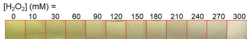
Figure S19. A composite image of solutions of compound 1 after exposure to hydrogen peroxide, viewed under ambient lighting ([ 1 ] = 10 \mu M in acetonitrile)
