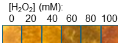
Figure S32. A composite image of Whatman #1 filter paper onto which compound 1 was adsorbed after exposure to H 2 O 2 vapors, viewed under 365 nm excitation
