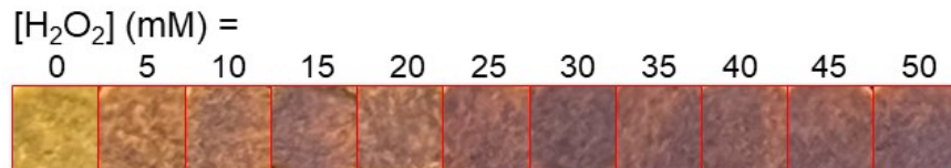
Figure S30. A composite image of Whatman #1 filter paper onto which compound 1 was adsorbed after exposure to hydrogen peroxide, viewed under 365 nm excitation
