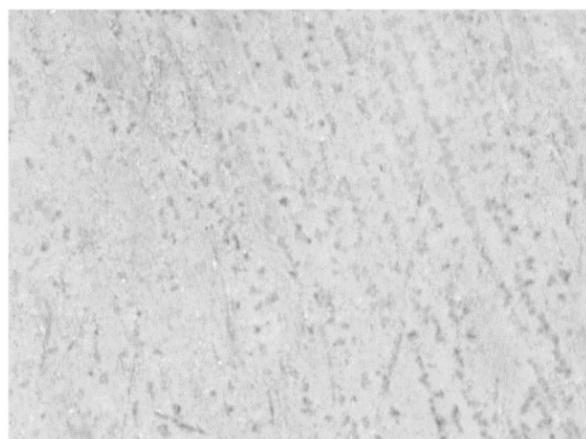
Figure S12: Optical image of the zinc surface after long-term cycling.
