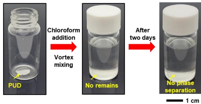
Fig. S11 Optical images of the PUD dissolution in the chloroform.
