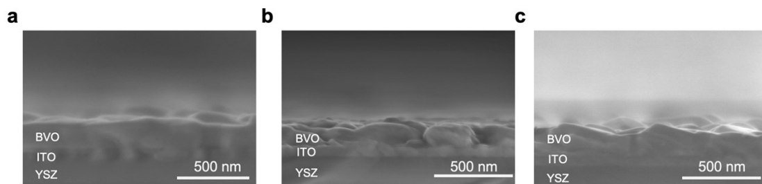
Figure S8. Cross-section SEM images of BVO thin film over YSZ (110) with two step deposition, under (a) 10 mTorr; (b) 20 mTorr; (c) 40 mTorr.
