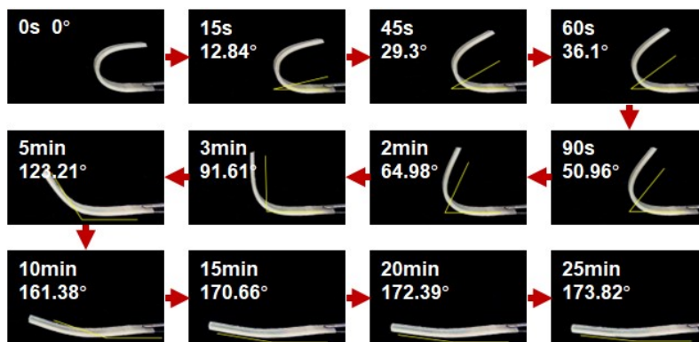
Fig. S8 Photographs of shape recovery performance of ATW at 40 °C within 210 s.
