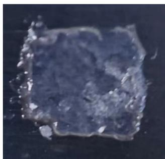
**Fig. S9** Photograph of LMA@PCC co-assembly after photo-curing under UV-365 light (175 W) for 5 min without trimethylolpropane triacrylate (The concentration of the PCC is  $2.0 \times 10^{-2} \text{ mol L}^{-1}$ ).
