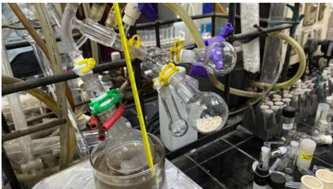
Fig. 1: Distillation setup after a scale-up reaction to recover the HFIP for reuse.
