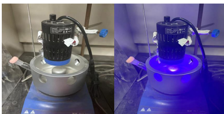
Figure S2. Photoreactor for Procedure B.
