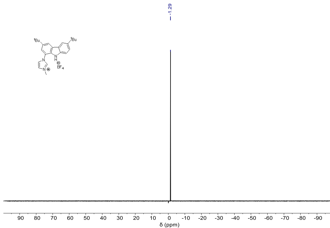
Figure S26. ^{11}\text{B}\{^1\text{H}\} NMR spectrum of 1-(3,6-di- tert -butyl-9 H -carbazol-1-yl)-3-methyl-1 H -imidazol-3-ium tetrafluoroborate in \text{DMSO-}d_6 at 160 MHz.
