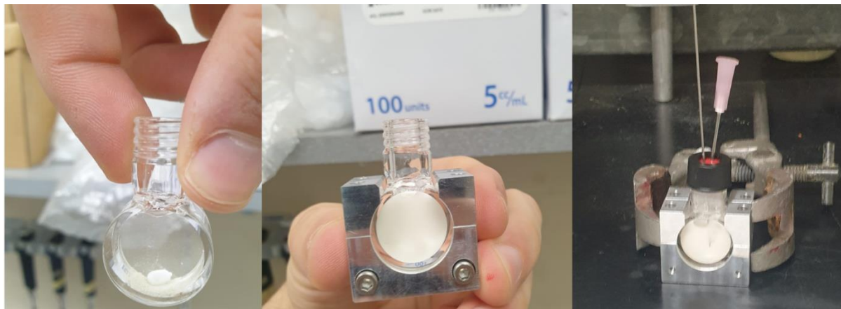
Figure S6: Photocatalysis reactor cell set-up; filling the photocatalyst, adding the water, and performing the purge by bubbling Ar through a needle.
