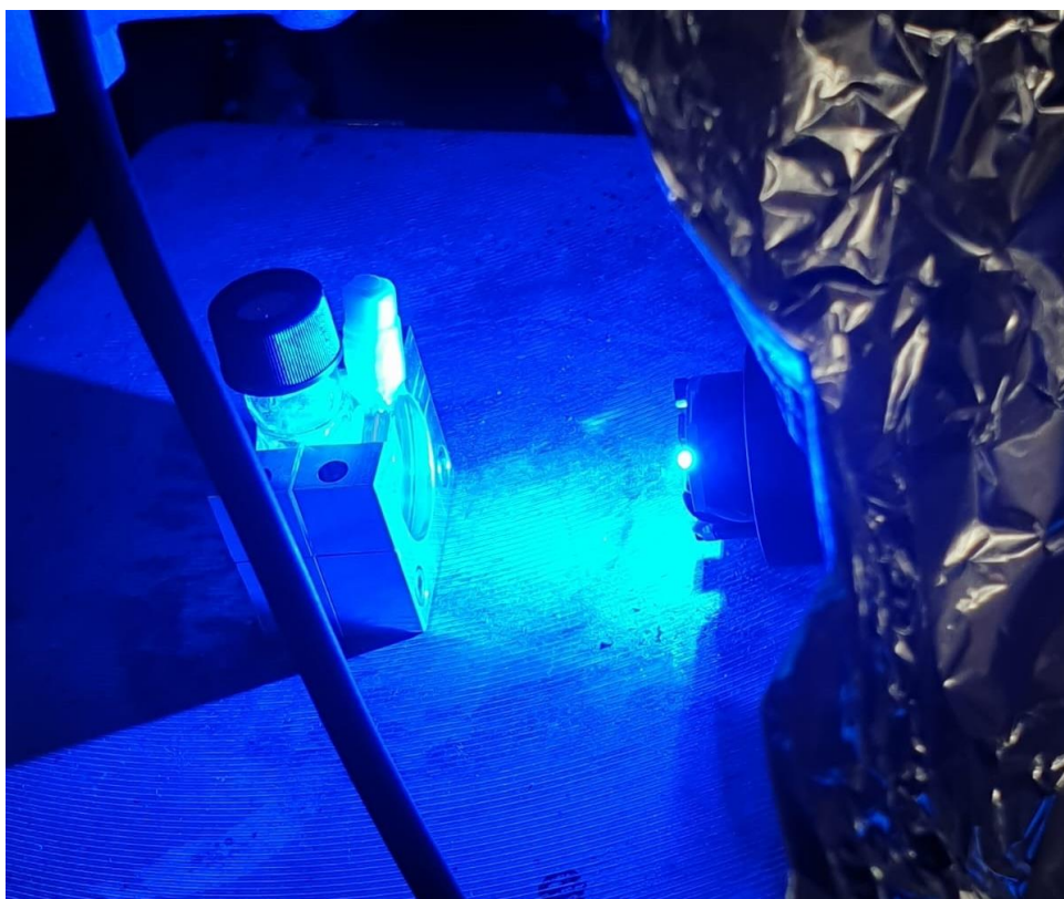
Figure S7: Photo showing the photocatalysis reactor in operation under 455 nm LED illumination. The metal support ensures the cuvettes containing the UC material and the photocatalyst material close together.
