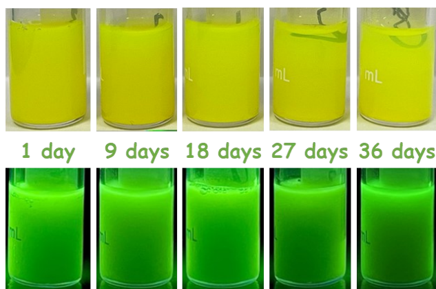
Fig. S6 Photographs of C_2P_3B_8 AQDs with PEG protection under natural (up) and UV light irradiation at 365 nm excitation (down) with time goes.
