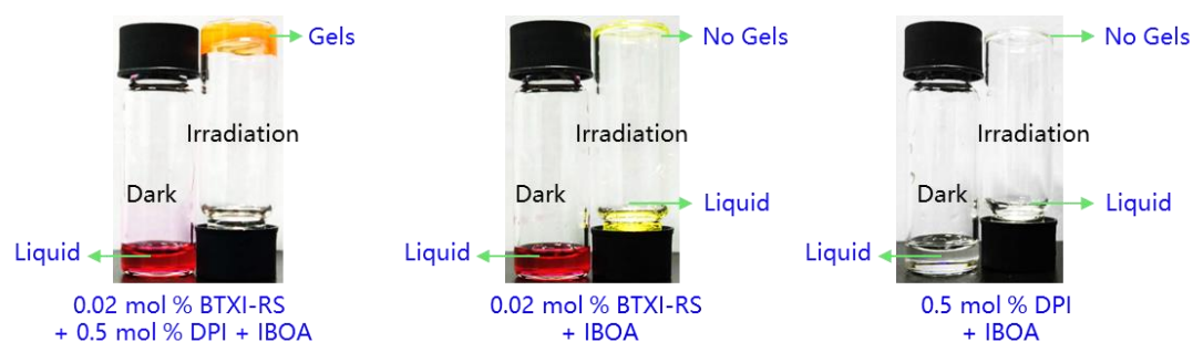
Figure S51. The experiment for the polymerization of monomer (IBOA), conditions: BTXI-RS , diphenyliodonium salt, irradiated for 5 minutes with the wavelength of optical fiber is 532 nm ( 100 \text{ mW cm}^{-2} ).
