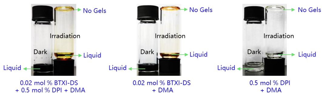
Figure S46. The experiment for the polymerization of monomer (DMA), conditions: BTXI-DS , diphenyliodonium salt, irradiated for 5 minutes with the wavelength of LED is 630 nm ( 100 \text{ mW cm}^{-2} ).
