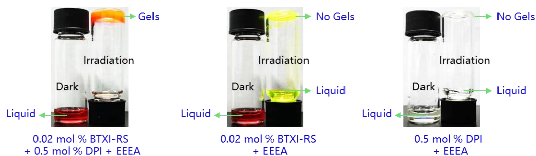
Figure S50. The experiment for the polymerization of monomer (EEEA), conditions: BTXI-RS , diphenyliodonium salt, irradiated for 5 minutes with the wavelength of optical fiber is 532 nm ( 100 \text{ mW cm}^{-2} ).
