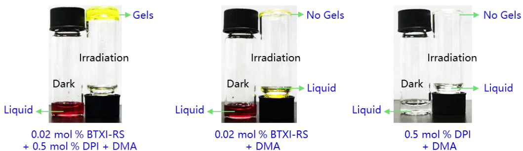
Figure S49. The experiment for the polymerization of monomer (DMA), conditions: BTXI-RS , diphenyliodonium salt, irradiated for 5 minutes with the wavelength of optical fiber is 532 nm ( 100 \text{ mW cm}^{-2} ).
