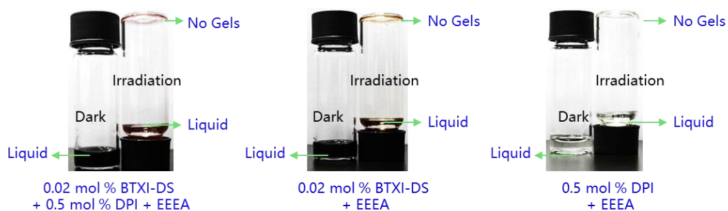
Figure S47. The experiment for the polymerization of monomer (EEEE), conditions: BTXI-DS , diphenyliodonium salt, irradiated for 5 minutes with the wavelength of LED is 630 nm ( 100 \text{ mW cm}^{-2} ).
