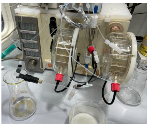
Figure S6. Representative Vapourtec equipment used in temperature-driven condensation reaction
