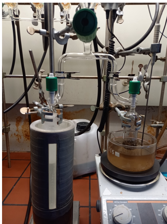
Figure S25. Experimental setup for the direct synthesis of \text{PCl}_3 directly from \text{P}_4 and [\text{NEt}_3\text{Me}][\text{Cl}_3] .
