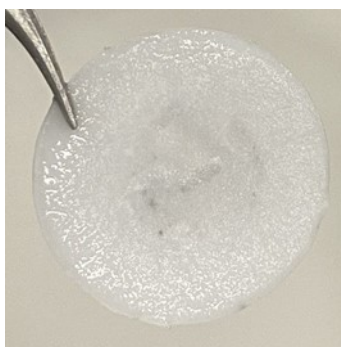
Figure S5. A photograph of the glass filter in a \text{Na}/\text{Na}_{2/3}\text{MnO}_2 cell with 5 M NaFSA in DME electrolyte after 200 cycles in the voltage range of 1.5–4.0 V at a rate of 50 \text{ mA g}^{-1} .
