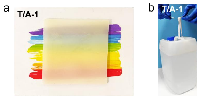
Figure S3. (a) The photograph of T/A-1. (b) The T/A-1 failed by brittle fracture without lifting the weight.
