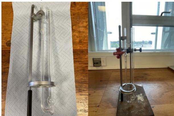
Figure S5.1: Photographs showing the Micro-Ostwald viscometer used to determine the viscosity of \text{Li}[\text{B}(\text{hfiP})_4] \cdot 2\text{DME} ( 1a -2DME), \text{Li}[\text{Al}(\text{hfiP})_4] \cdot \text{DME} ( 1b -DME) and \text{Li}[\text{Al}(\text{hfiP})_4] ( 1b ).
