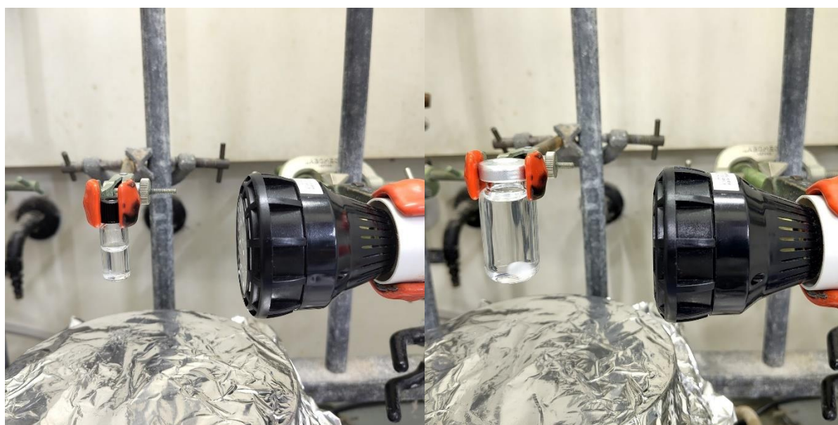
Figure 3: Reaction set up before illumination. On the left: for 0.1 mmol scale. On the right: for 1 mmol scale
