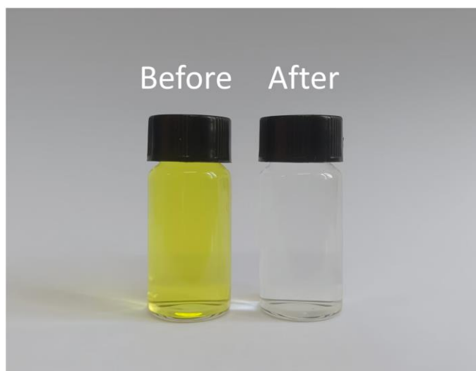
Fig. S17 Color change of the recovered electrolyte before and after reaction.
