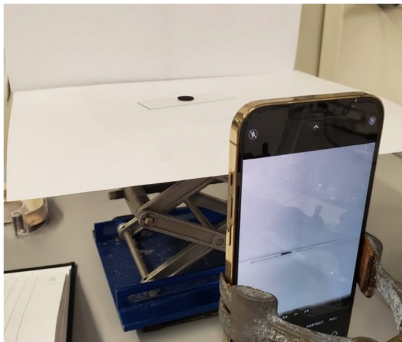
Figure S15 Surface contact angle experimental setup
